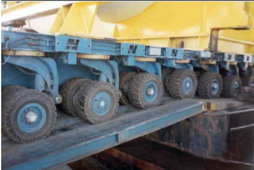
Figure 2: Roll on to barge using hydraulic axles. (Macsween, 2004)
