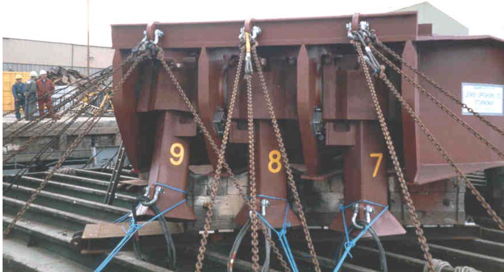
Figure 7: Typical lashing arrangement. (Macsween, 2004)
