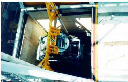
C) Launching the ROV through moon pool on a boat
