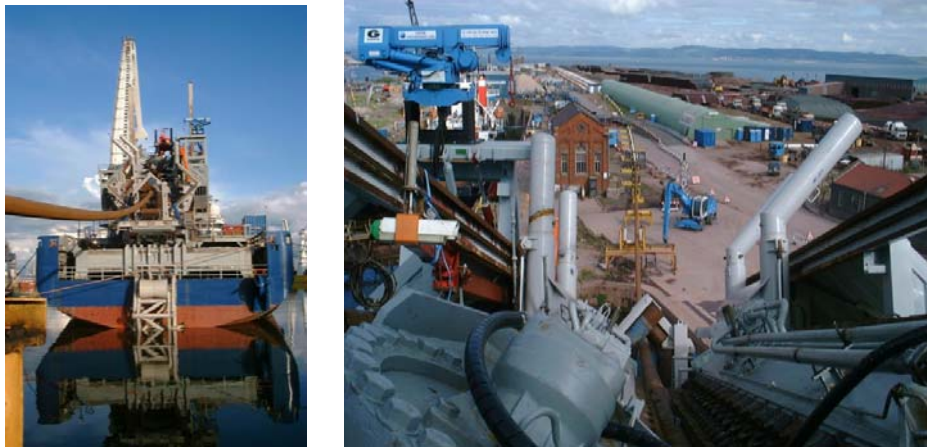
Figure 9-5 Pipe Spooling onto Pipelay Vessel - Scandi Navica Subsea 7 Vessel
