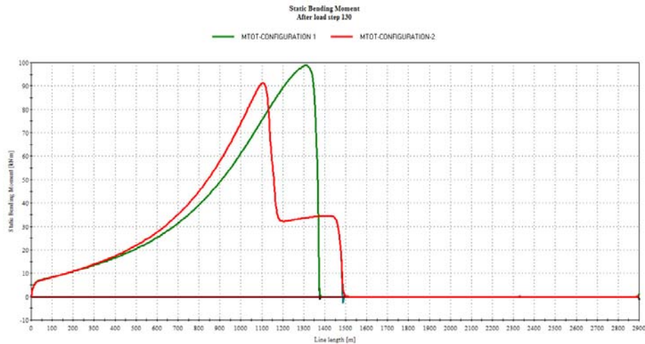
Figure 5-11 Static Bending Moments – Configuration 1 & Configuration 2 (Mean Case)
