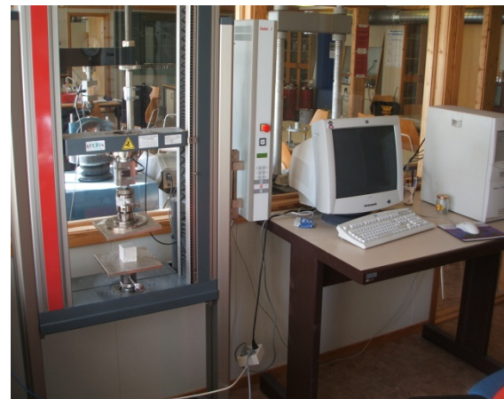
Figure 7: Material testing machine Z020/TH2S, Zwick 2001
