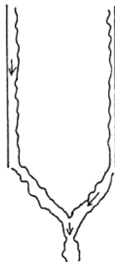
Figure 2.19 Unvented vertical pipe expelling to atmosphere at low flow rate (Thorpe et al., 1989).
