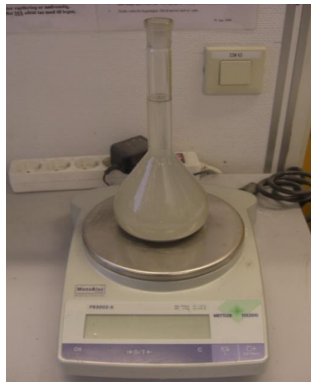
Figure 2: Volumetric flask filled with aplite and water up to the 1000 ml line.
