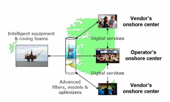
Figure 1-4. Concept of Integrated operations (OLF, 2003)
