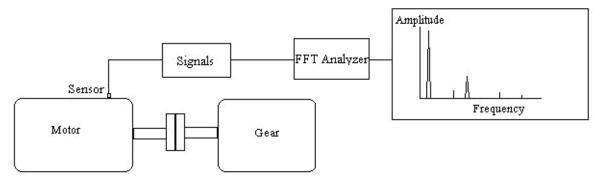
Figure 2-8. Vibration Monitoring
