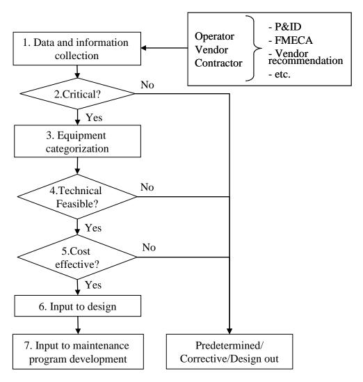
Figure 5-2. Methodology for selecting equipment suitable for CBM.
