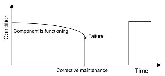
Figure 2-5. Corrective Maintenance
