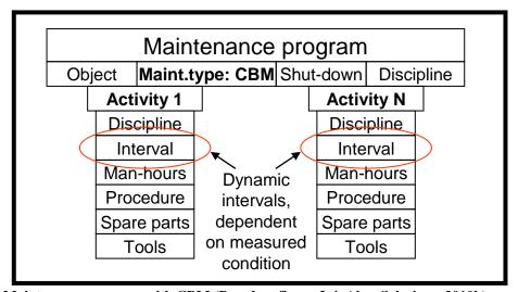
Figure 5-6. Maintenance program with CBM (Based on figure 2-4, Aker Solutions, 2010b)
