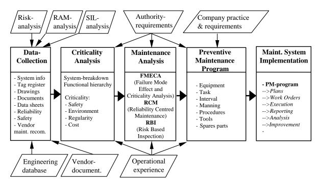
Figure 2-2. Maintenance engineering work process (Aker Solutions, 2010b)
