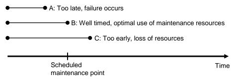
Figure 3-2. Timing of scheduled maintenance with respect to failures (Markeset, 2008)
