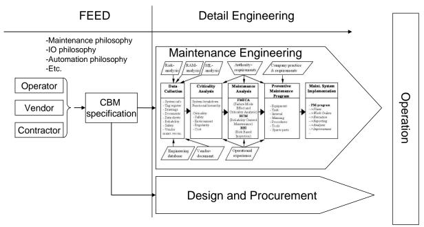
Figure 5-1. CBM engineering work process.
