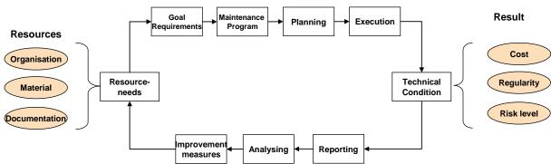
Figure 1-1. Maintenance management process (NPD, 1998)
