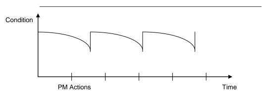
Figure 2-6. Predetermined Maintenance
