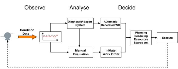
Figure 2-7. Condition Based Maintenance work process (Aker Solutions, 2009)
