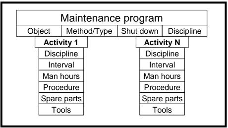
Figure 2-4. Typical maintenance program content (Aker Solutions, 2010b).
