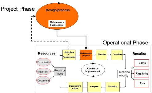
Figure 1-3. Project phase in the maintenance management process (Aker Solutions, 2010b)
