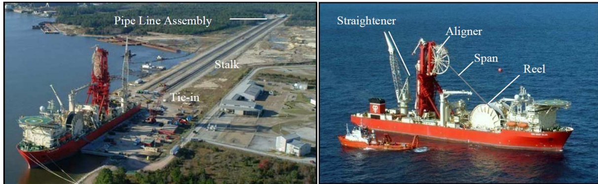
Figure 6-5 Spooling and Lay Phase [Denniel, 2009]
