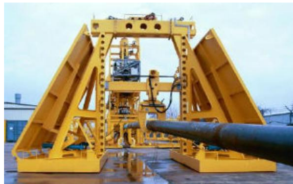
Figure 9-6. Pipe Lifting Frame (OTC 16635).
