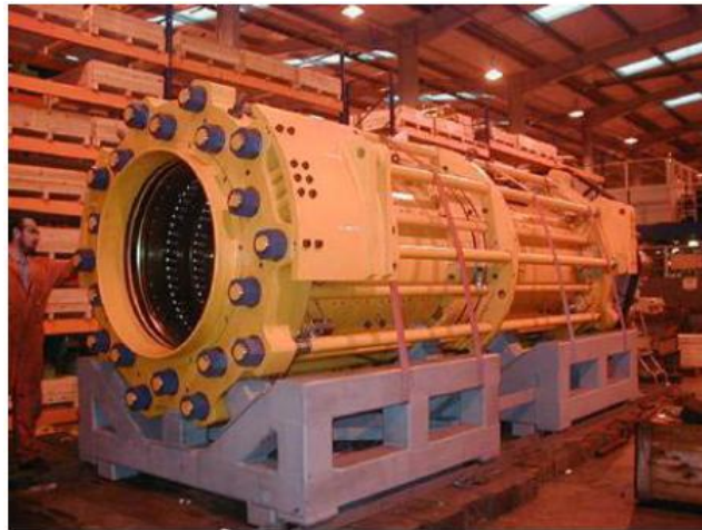
Figure 6-11. Morgrip connector (source: Hydratight)
