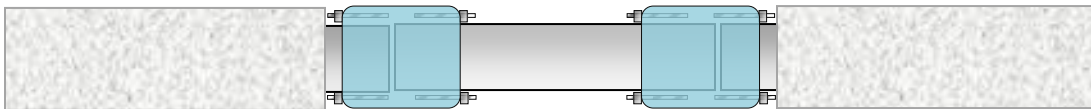
Figure 2-4. Mechanical couplings fix the pipe spool to the mainline and restore the integrity.
