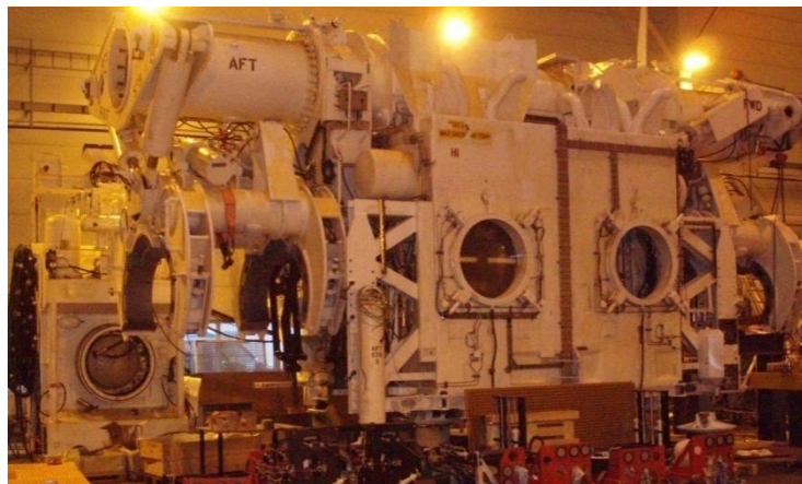
Figure 6-15. Dry habitat with the diver access and assistance (courtesy of Statoil).
