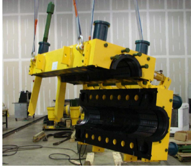
Figure 7-2. Opened clamp (source: OTC19207).
