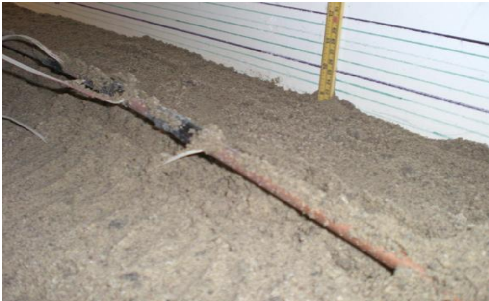
Upheaval buckling simulation from an experiment
