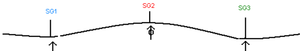
Figure 7.9 Curvature variation post max force
