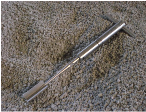
Figure 5.7 Geonor H-60 hand-held vane tester
