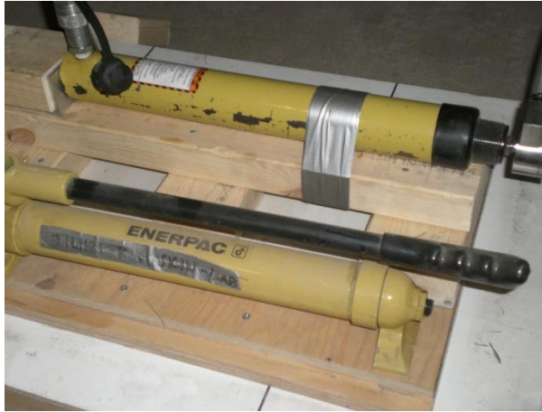
Figure 5.1 Enerpac hydraulic cylinder and jack
