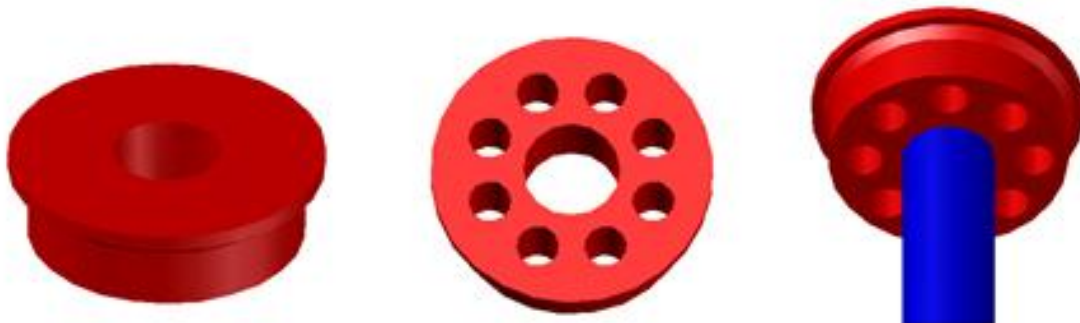
Figure 4-1: The top-hat as intended to the left while redesigned with holes in the middle and to the right.
