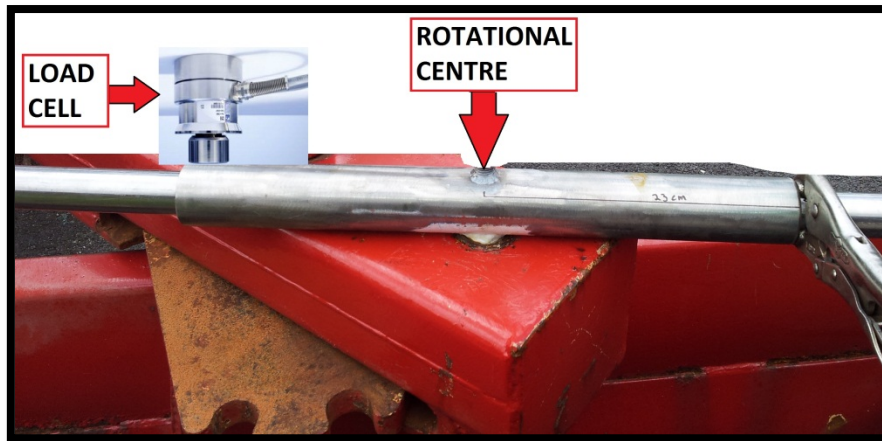
FIGURE 5-12 LOAD CELL PRINCIPLE
