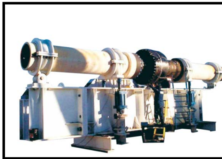
FIGURE 2-10 TESTING RIG OF A CONNECTOR (GE ENERGY, 2012)
