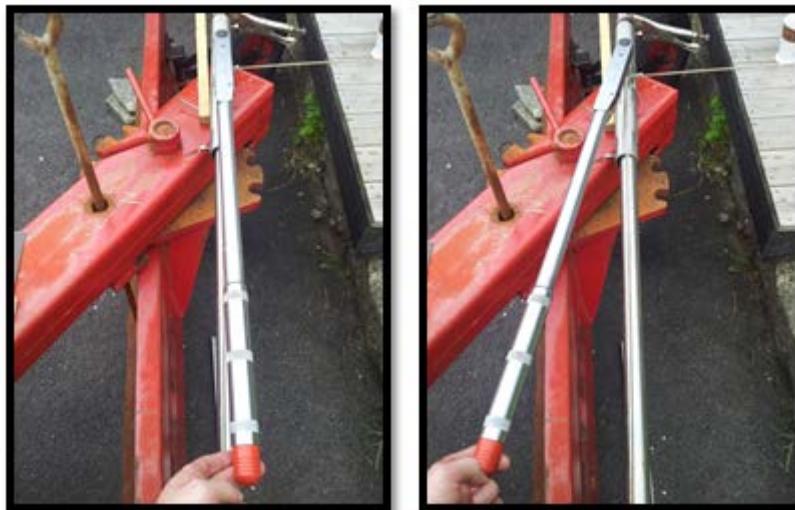
FIGURE 5-7 PLAY BETWEEN BOLT AND WRENCH
