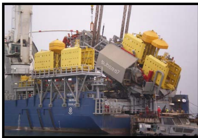
FIGURE 2-6 PIPELINE END TERMINATION - PLET (BP NORWAY, 2012)
