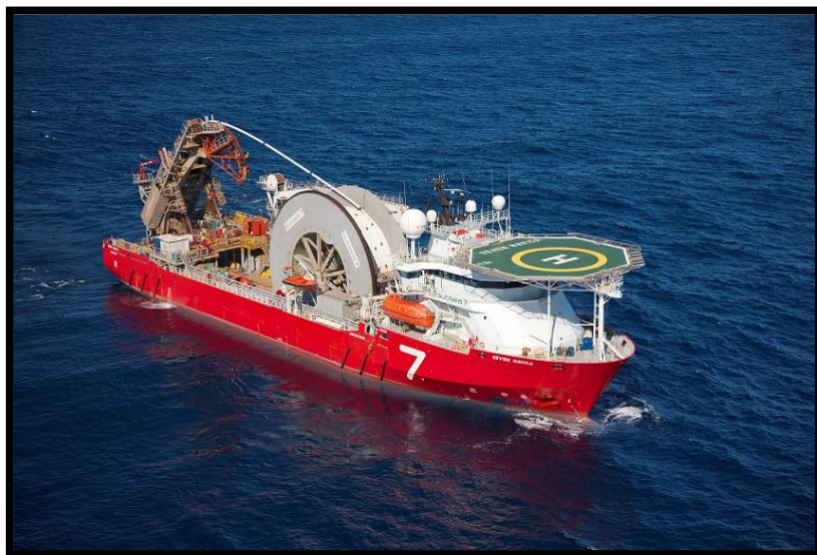
FIGURE 2-4 SUBSEA 7'S REEL LAY VESSEL SEVEN NAVICA (ENGINEER LIVE, 2012)
