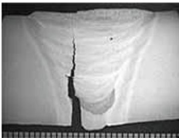
Figure 10 H 2 S Corrosion crack and pressure build up [Hatton, S., 2010, HTHP]
