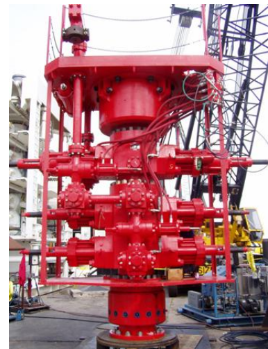
Figure 4 A Blowout Preventer, Credit: Cameron-Nutronix [The Encyclopedia of Earth, 2012]
