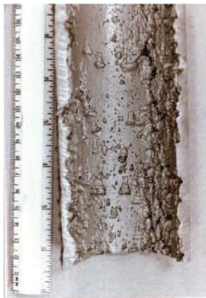
Figure 9 Heavy pitting and general wall loss [Hatton, S., 2010, HTHP]
