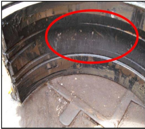
Figure 6 Eccentric wear to the packer element [Upton, T.L., 2009]
