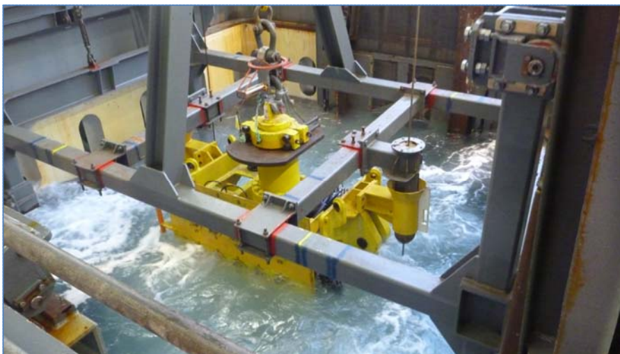
Figure 2.10 Cursor frame support subsea equipment lifted through moonpool (Heng, 2012)
