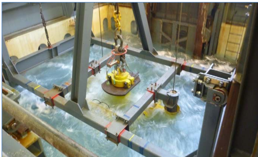
Figure 2.19 Subsea equipment getting lowered through moonpool splash zone (Heng, 2012)
