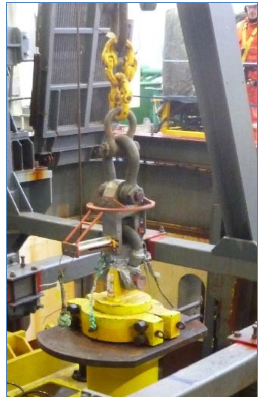
Figure 2.5 Moonpool lift - rigging configuration (Heng, 2012)
