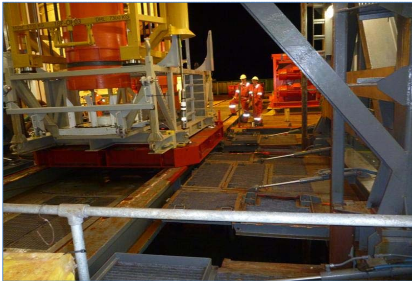
Figure 2.17 Skidding of subsea equipment (Heng, 2012)
