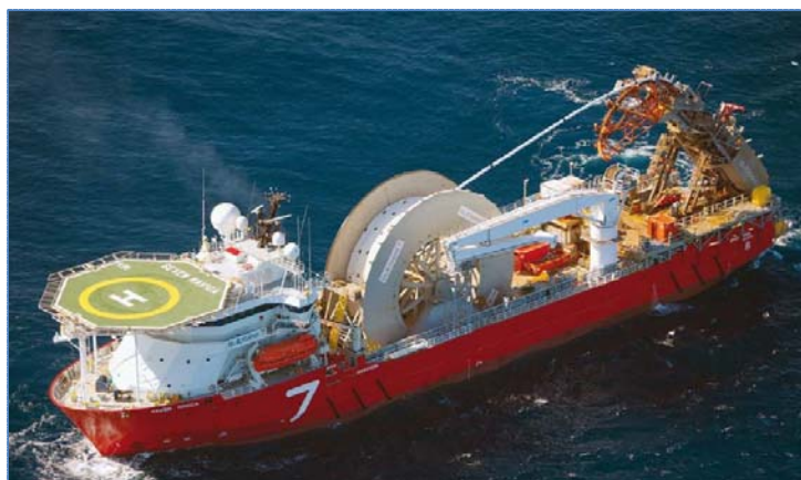
Figure 2.1 Seven Navica performing a reel pipe-lay (Subsea 7, 2011)
