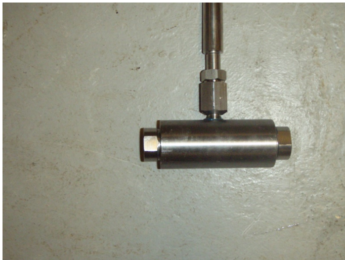
Figure 6.5: Pressure vessel (Bridgman's chamber) connected to high pressure hose
