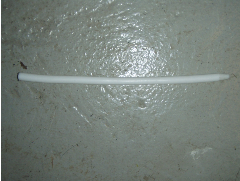
Figure 6.6: PTFE rod after test, a close look will show the initiated yielding and reduction of the outer diameter
