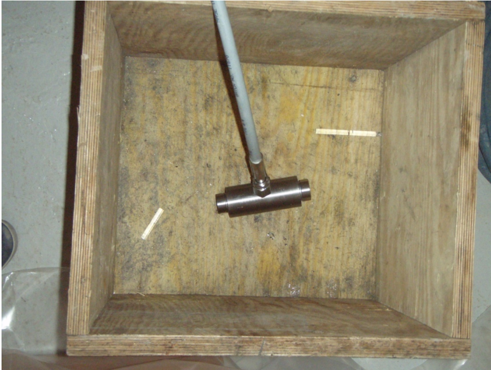
Figure 6.9: Pressure vessel and ruptured rod parts inside a wooden crate
