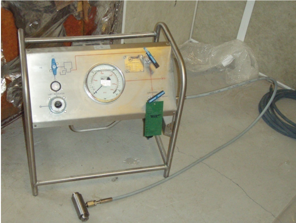
Figure 6.8: High pressure unit connected to the pressure vessel
