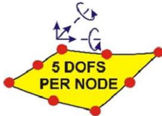
Figure 5: Thin shell element.
