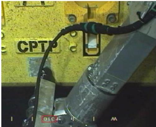
a) ROV-operated probe
