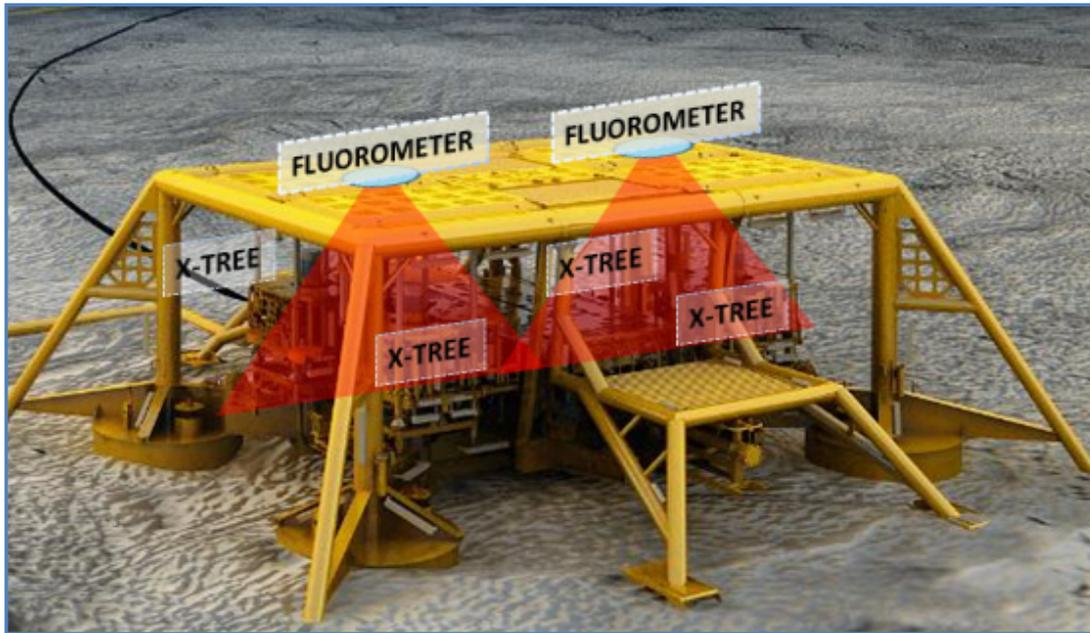
Figure 4-5- Fluorometers installed on subsea template
