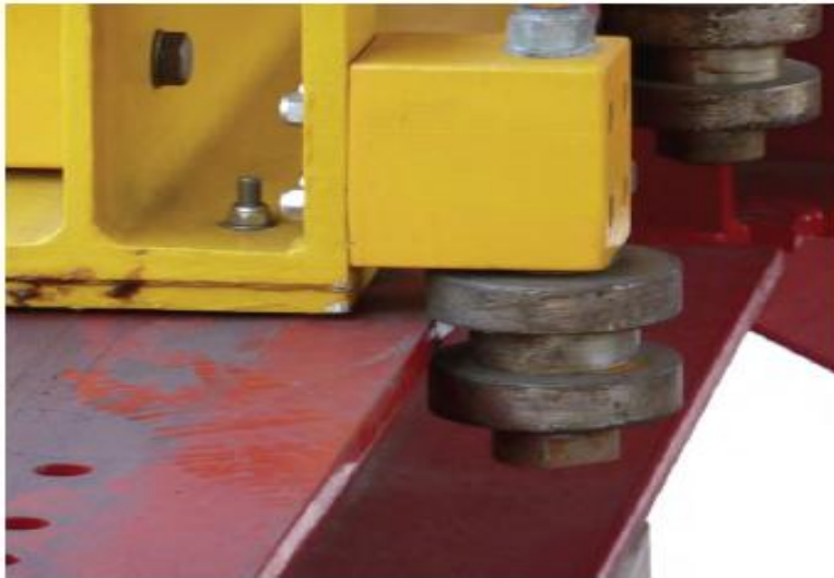
Figure 14: Too much clearance on the rollers
