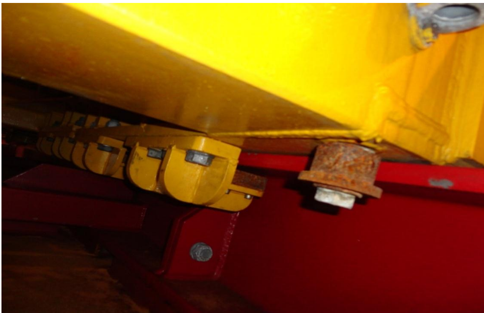
Figure 35: Rollers and skidding arrangement under the pallet
