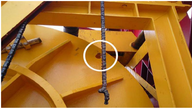
Figure 28: The hole on the drum used for lifting the main winch
