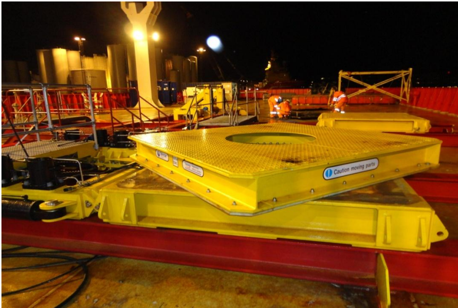
Figure 34: Trolley on the skidding beams
