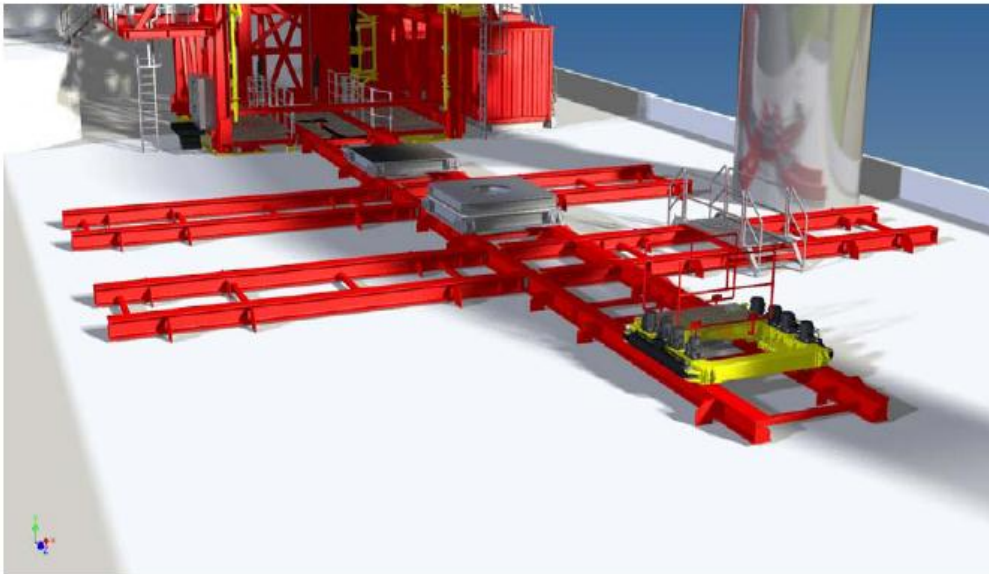
Figure 5: Skidding system level 1
