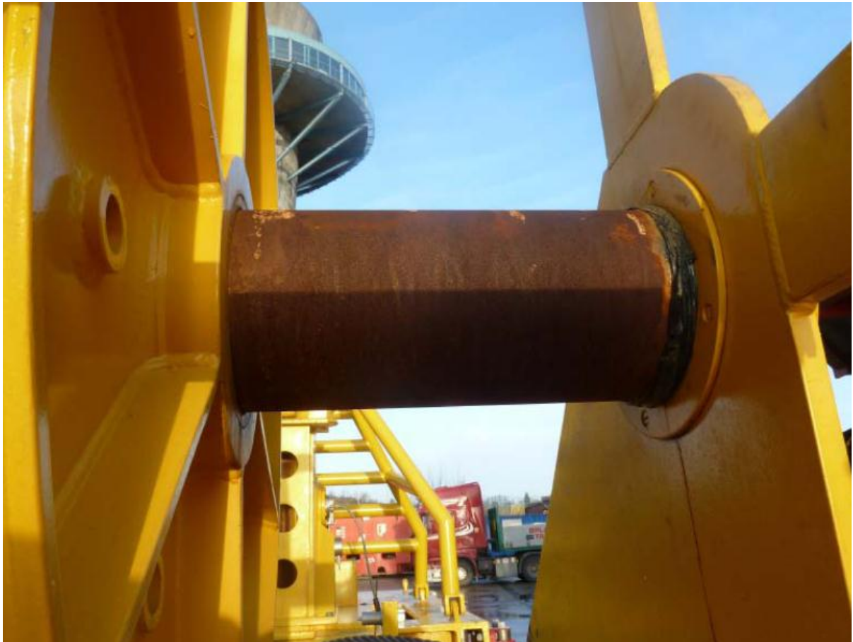
Figure 22: Corrosion of shaft
