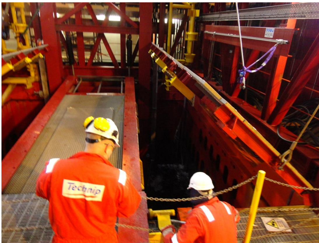
Figure 40: Moon pool doors partly opened
