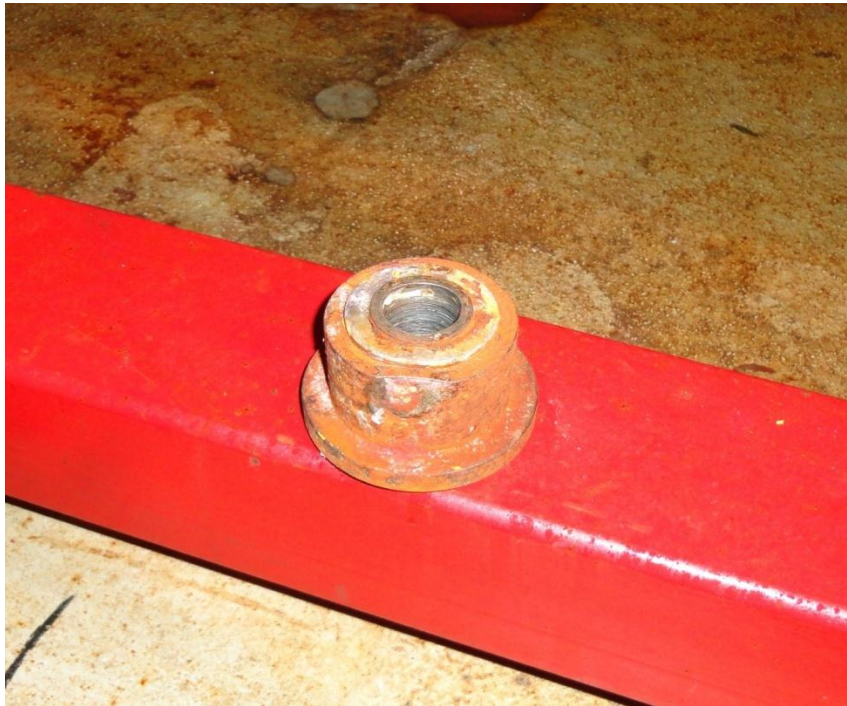
Figure 36: Broken bearing on deck
