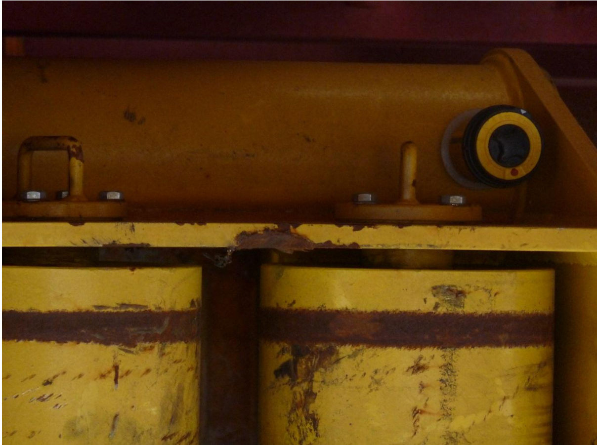
Figure 26: Spooler damaged by wires
