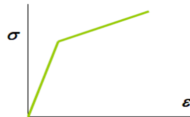
(c) Piecewise linear (strain-hardening) material.
