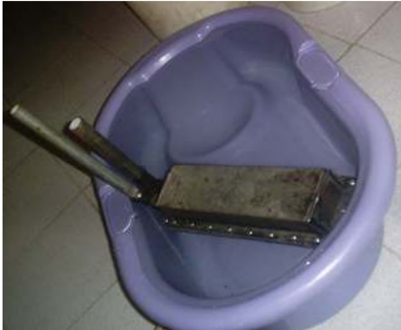
Figure-4.3: Checking the equipment for leaks (12hrs)
