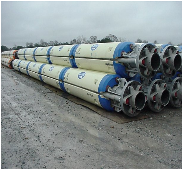
Figure 2.5 Drilling riser joints with buoyancy modules [51]
