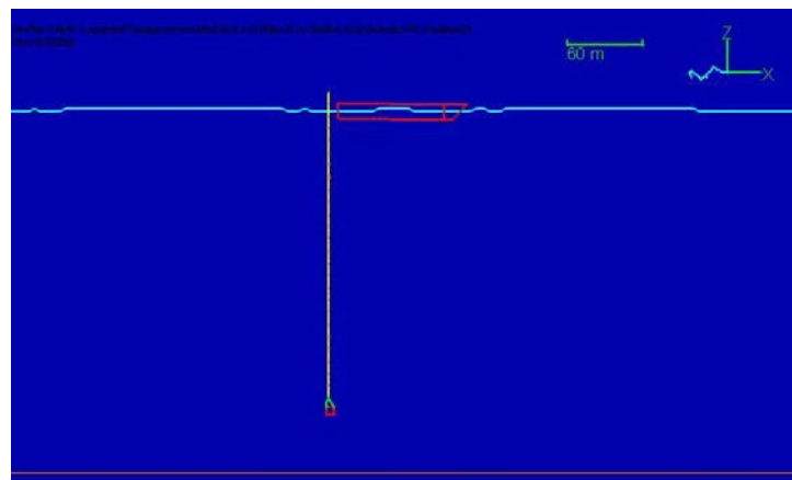
Figure 6.4 Sample for Lowering a subsea package [23]
