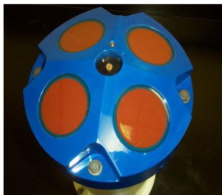
Figure 8.4 Head of an ADCP with the four transducers [34]
