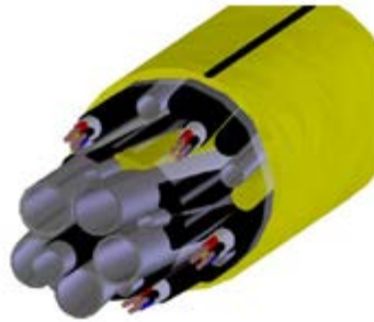
Figure 4.5 Steel Tube umbilical [22]
