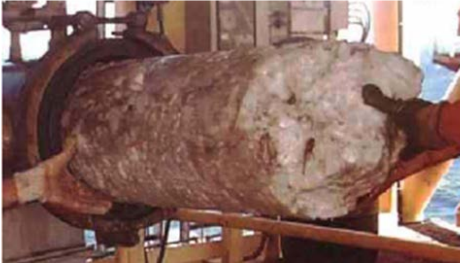
Figure 2.3 Hydrate removals from pipeline [47]
