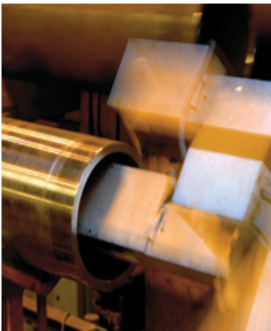
Figure 2.8 Laser End Measurement Systems [53]
