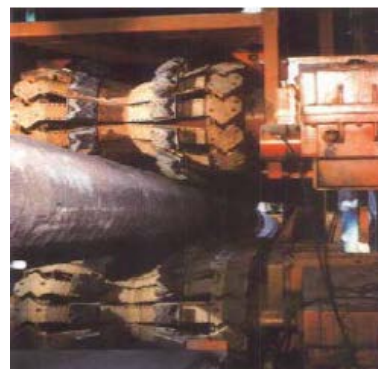
Figure 5.3 Typical tensioner used for S-Lay [15]
