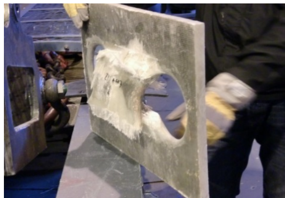
Figure A.8: Ultimate failure mode of Case 2.
