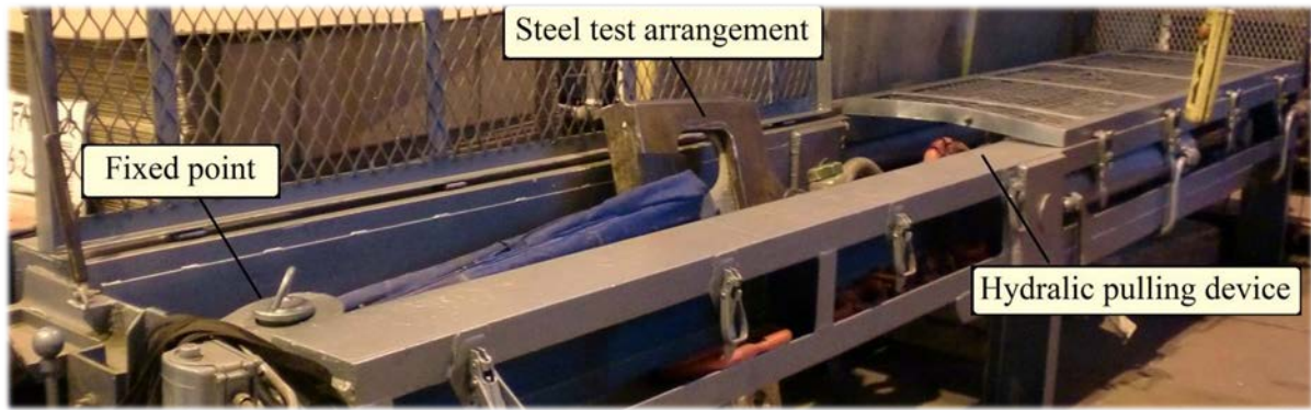
Figure 4.1: Hydraulic tensile bench with the Case 3 test setup.
