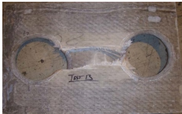
Figure A.5: Case 1 ultimate failure
