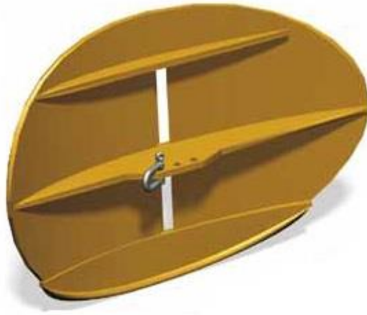
Figure 2-6 An illustration of a typical oval shaped Otter door[6]
