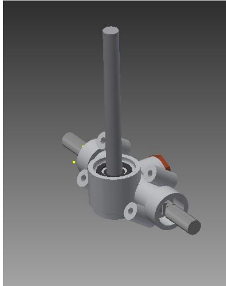
Figure 6-2: Aluminium steering rack from IC-Kart
