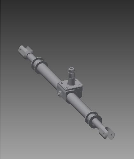
Figure 6-1: Carbon fiber steering rack from Formula Seven
