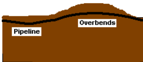
Figure 1 - Pipeline with overbend
