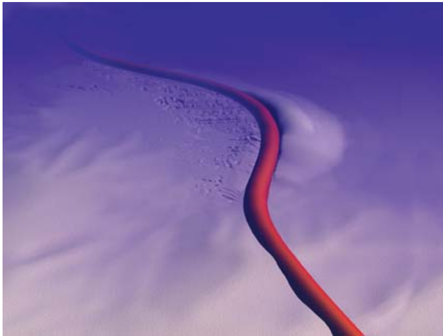
Pipeline exposed to lateral buckling 20
