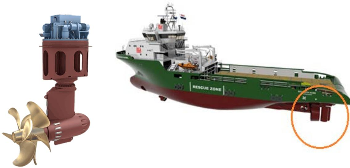
Figure 9: The main propulsion thruster
