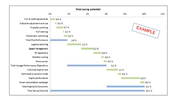
Figure 6: An example of an specific energy saving potential
