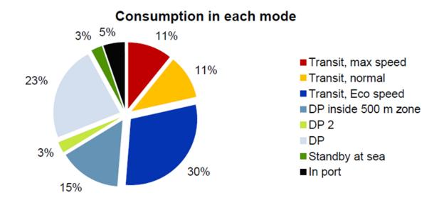
Figure 7: The specific operational mode consumptions
