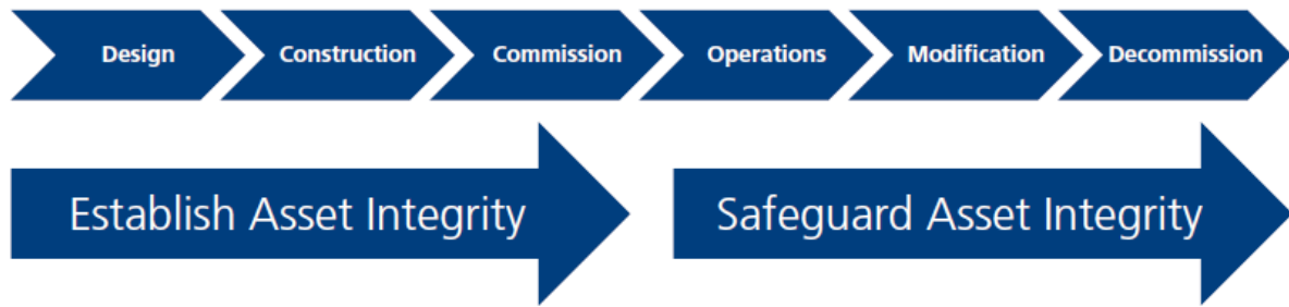
Figure 1.2: AIM Concept in the Lifecycle of an offshore Asset (Intertek, 2011).
