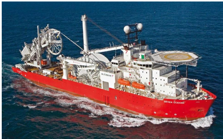
Figure 1.1 Reel Lay Pipeline Installation Vessel – Seven Oceans [31]
