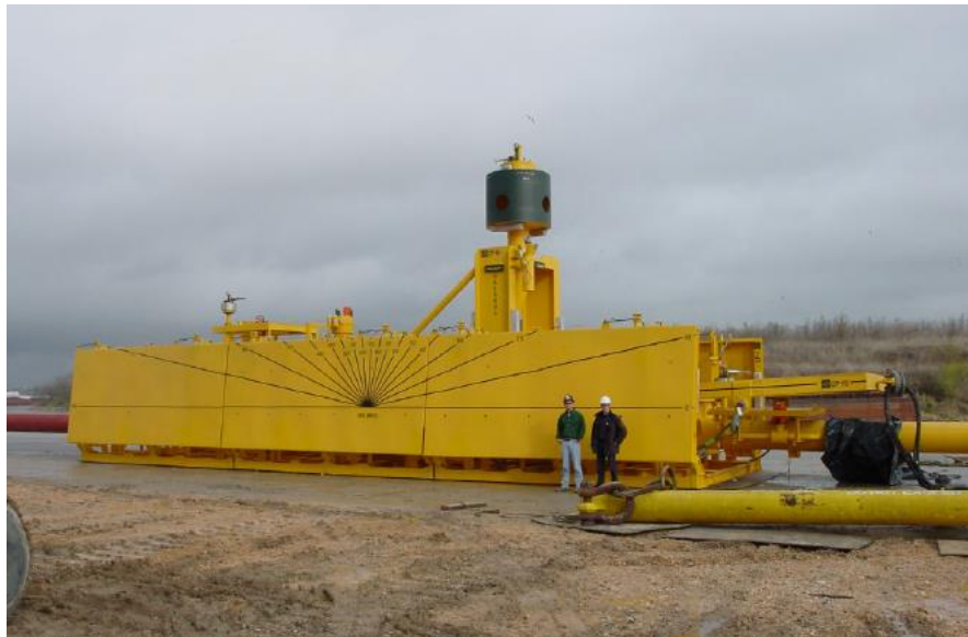
Figure 1.2 Very Large Inline Sled [28]
