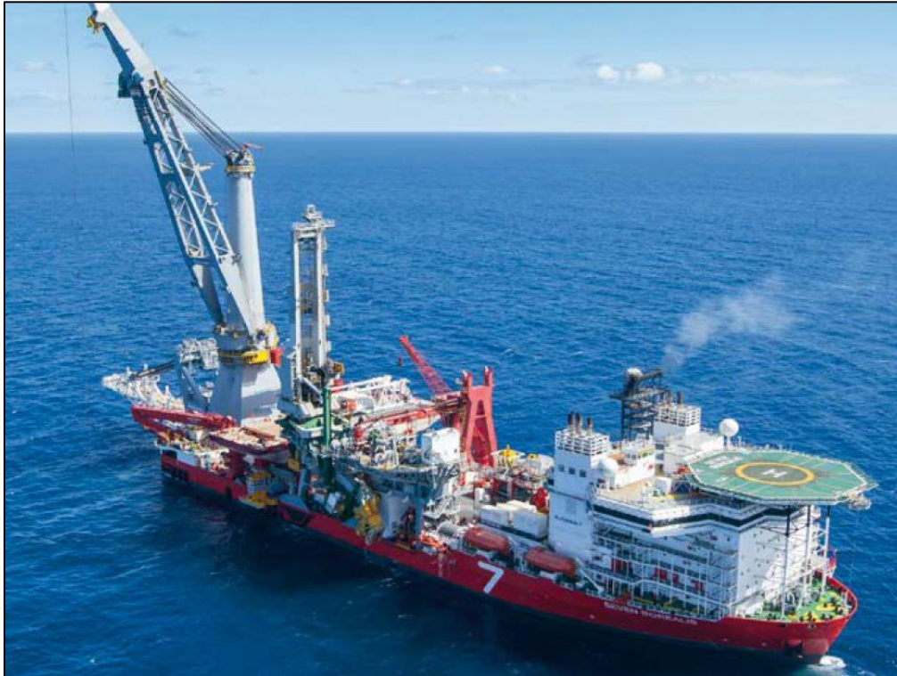
Figure 3.9 S and J Lay Installation Vessel – Seven Borealis [32]
