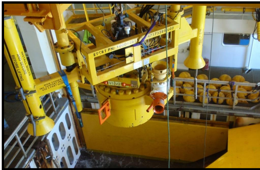
Figure 15 The ETC and ETCRT being lowered down into the moonpool
