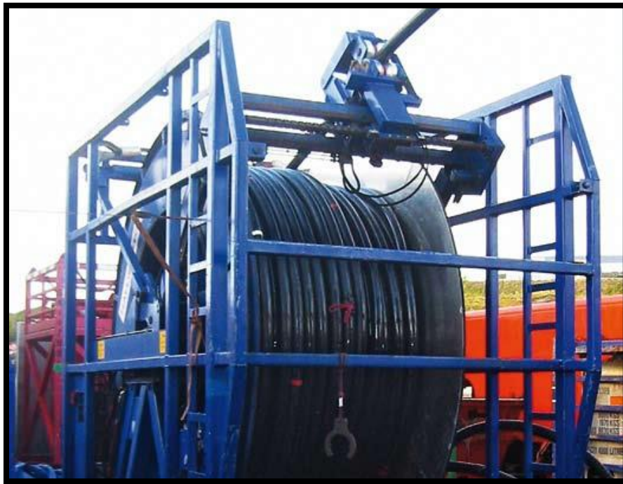
Figure 18 Picture of Black Eagle hose on a reel with a winch system (Offshore Magazine, 2011)
