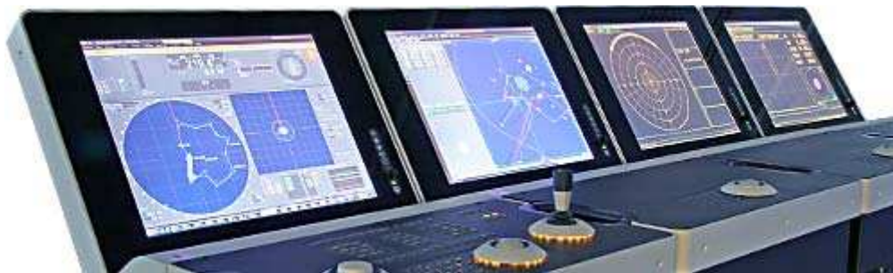
Figure1 Control station of Kongsberg DP system
