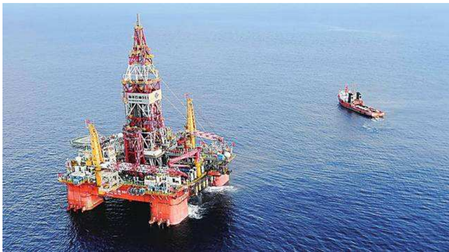
Figure 6-2 The sixth generation of semi-submersible drilling rig 'ocean oil 981' (Ref: http://szb.xgrb.cn:9999/epaper/xgrb/html/2012/05/08/03/03_76.htm )
