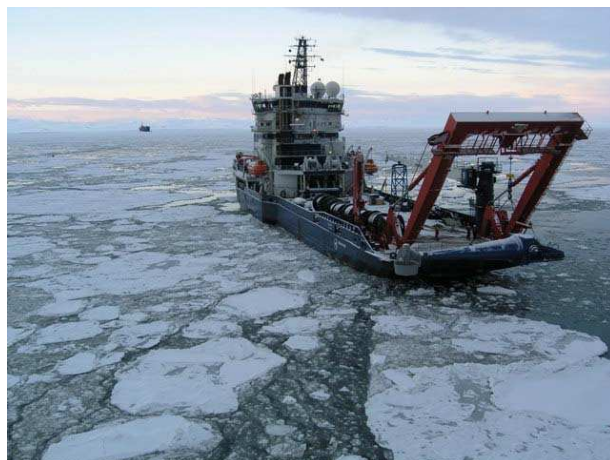
Figure 3-5 OSV conducts operation in ice covered area using DP system (Ref: Jensen et al., 2009)
