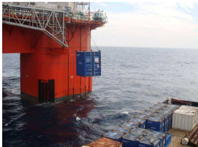
Figure3-3 Integrated DP operation between an OSV and a drilling rig
