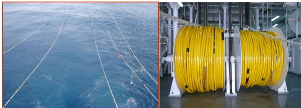
Figure 2. 6 Fluid filled streamer (left) and solid streamer (right) (credit: HYSY718 and HYSY720 GEO-COSL)
