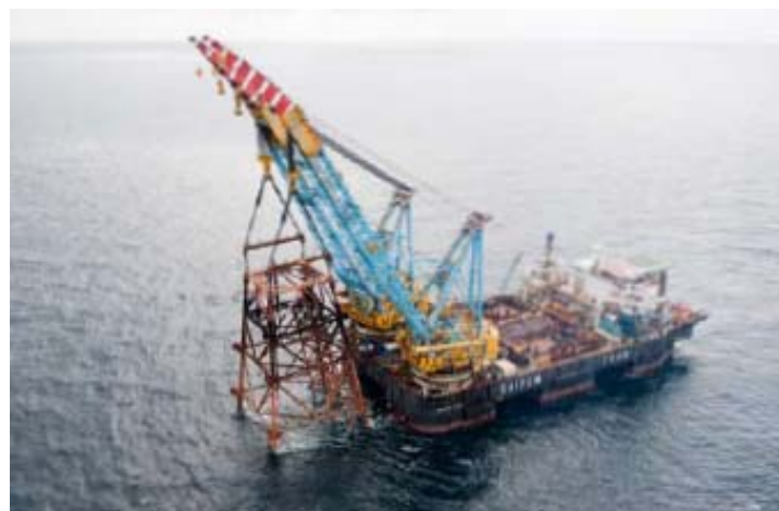
Picture 2-1 Transport of jacket using S7000 [24]
