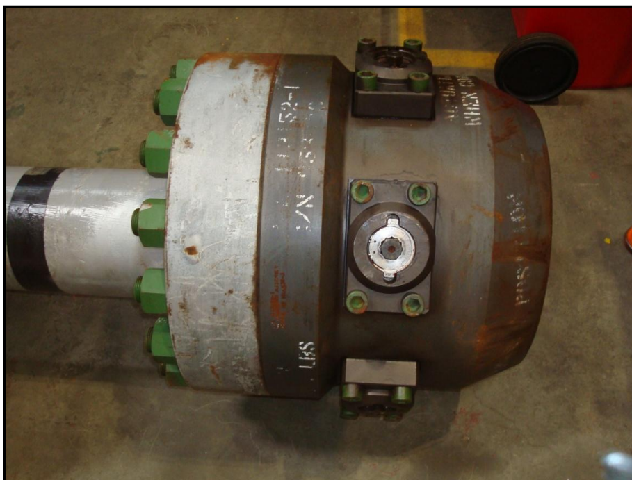
Figure 7-15 MR Connector at the bottom of stress joint
