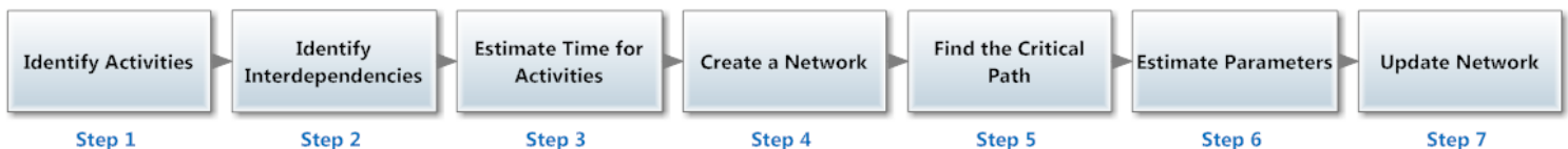
Figure 28 – The Critical Path Method flowchart (28)
