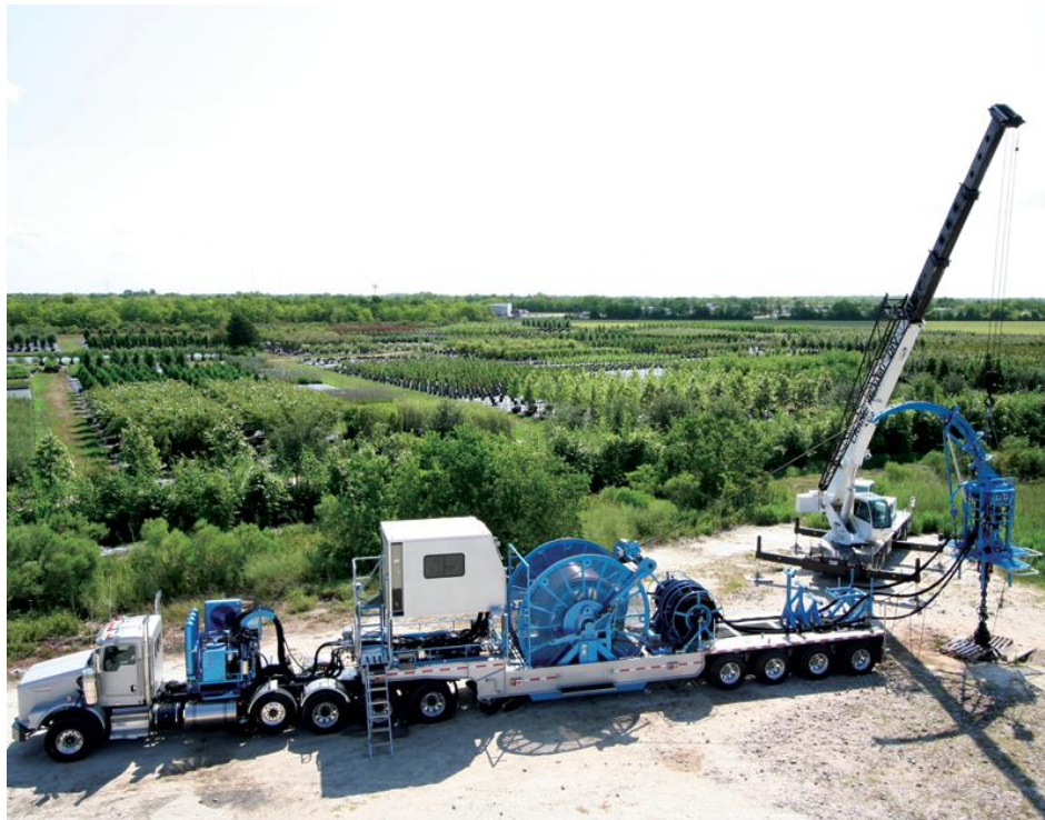
Figure 6 – Coiled Tubing unit (6)
