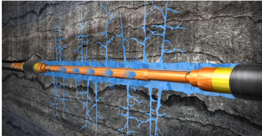
Figure 12 – Coiled Tubing Straddle Packer Method (12)
