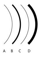
A) Thin film Epoxy (internal)B) Steel pipelineC) Anti corrosion coatingD) Reinforced concrete
