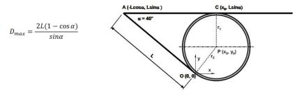
Figure 3-13 Anchor hooking size details (Tveit, 2011)
