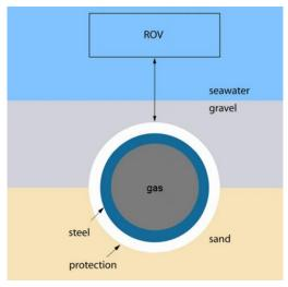
Figure 2-62 Pipetracker system (Fristedt and Silfverduk, 2009)
