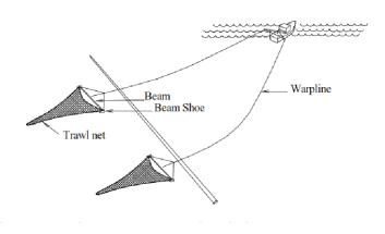
Figure 2-54 Typical beam trawl gear crossing a pipeline (DNV, 2010b)
