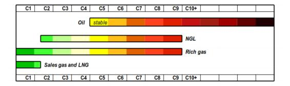
Figure 2-36 The basic hydrocarbon elements which encompass main different forms of pipelined natural gas (in addition to crude oil). (Odland, 2011)
