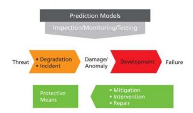
Figure 2-74 Figure 2 61 The development of a threat into a failure and the activities implemented to reduce the likelihood and/or consequences of such development (DNV, 2009)
