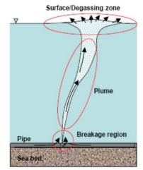
Figure 3-17 Illustration of gas leak from a ruptured subsesa pipeline (Gassco, 2007)
