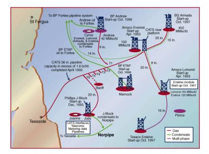
Figure 3-8 CATS pipelines (Pennwellnet, 2013)
