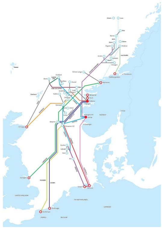
Figure 2-25 Norwegian natural gas pipeline infrastructure (Gassco, 2013)
