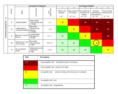
Figure 2-71 Risk matrix Source: DNV RP-116, integrity management of submarine pipeline systems
