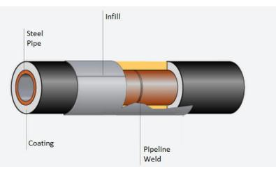
Figure 2-52 Field Joint. Source: (ASRO, 2009)
