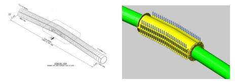
Figure 3-9 Sleeve solution BP CATS (Espiner, 2008)
