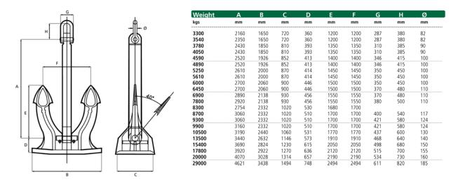
Figure 3-12 Stock Spek anchor specifications (Sotra, 2013)
