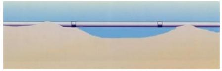
Figure 2-51 Free spans (FishSafe, n.d.)
