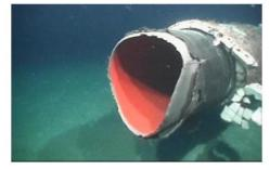
Figure 3-10 Transmed gilliotined pipeline (Orsolato, et al., 2011)
