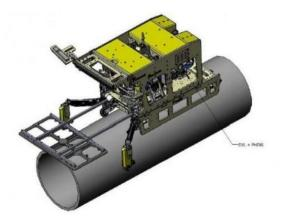
Figure 2-55 ROV General Visual Inspection (Oskarsson, 2012)
