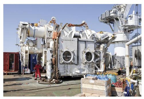
Figure 2-64 Statoil PRS Welding habitat (Nord-stream, 2013)
