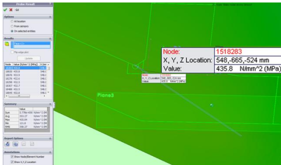
Figure B. 1: Maximum 1 st principle stress
