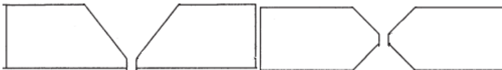
Figure 2: V-butt weld and X-butt weld (2)
