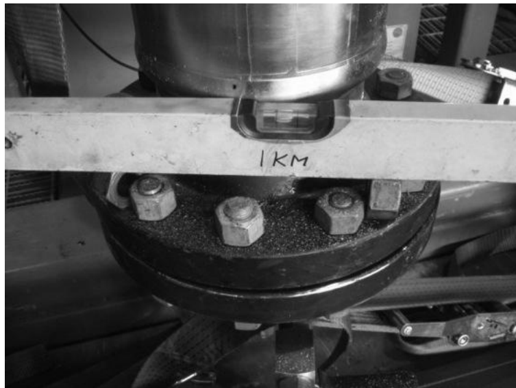
Figure 7.4 Bottom flange in level before loading
