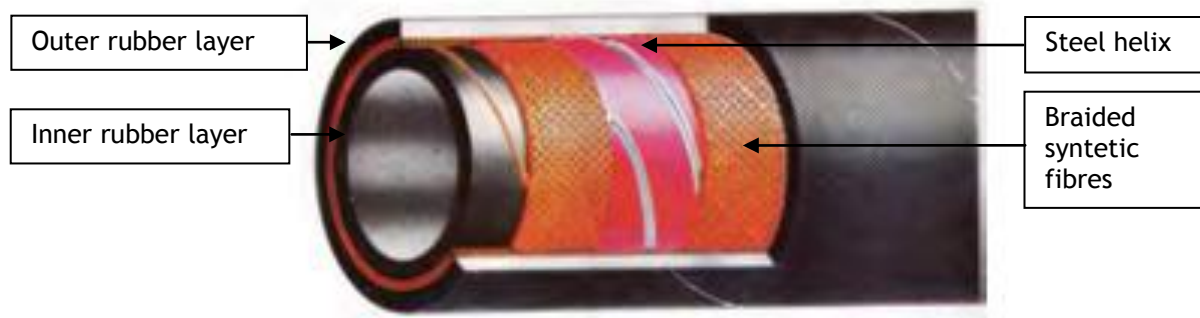
Figure 3.1 Oilflex Super build up layers [1]
