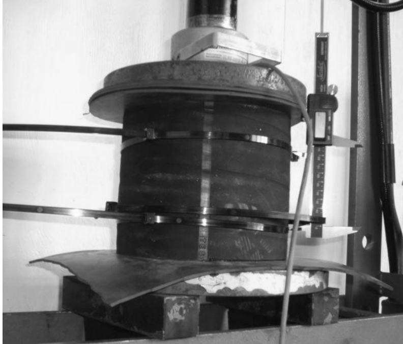
Figure 5.2 Close view of hose on test bench before loading sequence
