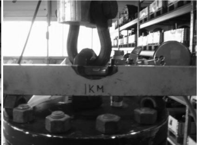
Figure 7.8 Top flange during lifting
