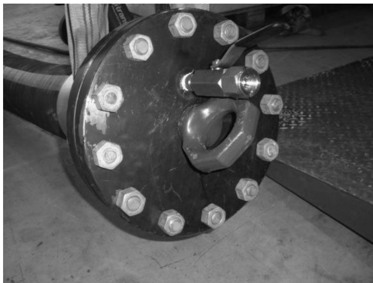
Figure 5.11 Close view of the bottom of the hose sample
