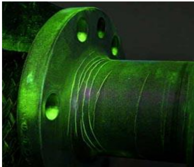
Figure 2.12 surface flaws detected by MPT (source: http://treborqs.com/services )
