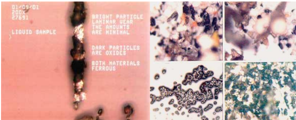
Figure 2.9 Particulate types distinguished by analytical ferrography (Beatty, 2004)
