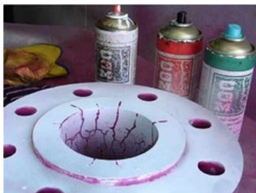
Figure 2.14 penetrant testing of a flange with cracks (Source: www.indiamart.com )
