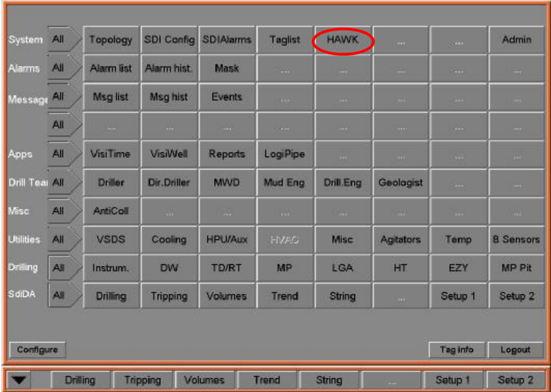
Figure 3.14 E-maintenance function embedded in Cyberbase systems
