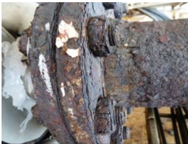
Figure 22: Picture of general rust build-up ca.10mm along the line
