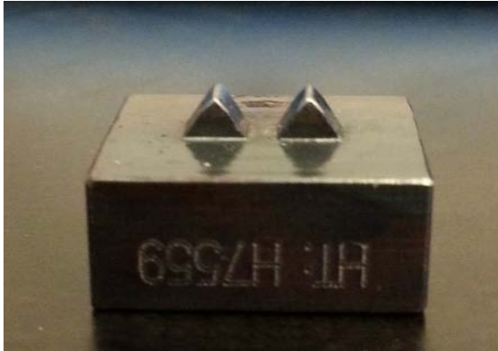
Figure 41: Double wedge 60° after testing with increased load. [2]
