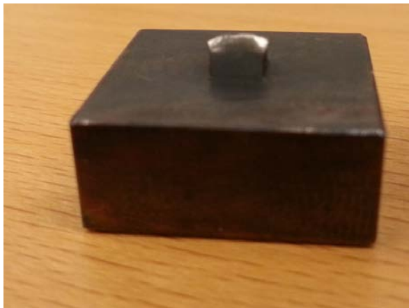
Figure 31: Wedge 60° indenter after testing with increased loading.[2]
