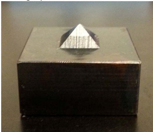
Figure 45: Pyramid indenter after testing with increased loading.[2]
