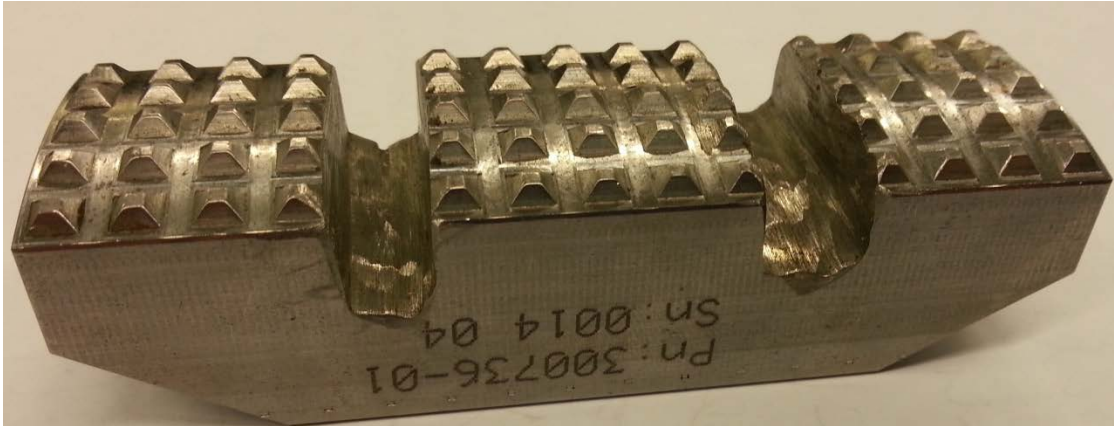
Figure 2: A slips element prototype that was tested on the TorcPlug®.[2]
