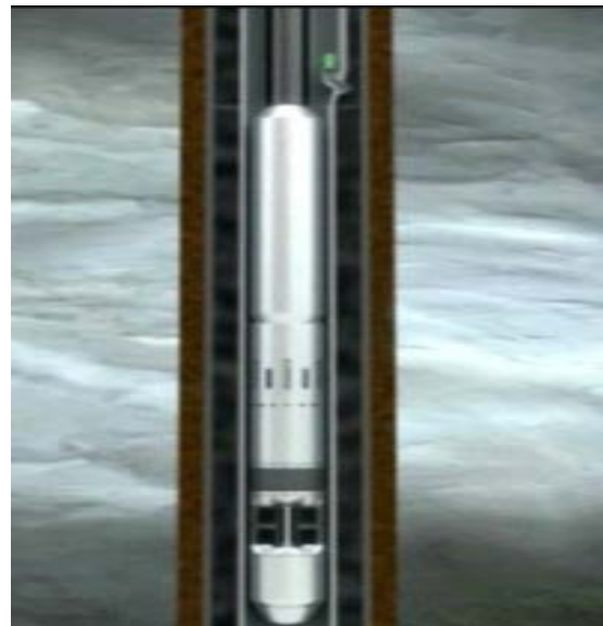
Figure 1: TorcPlug® in iso view and its placement inside the production tubing.[1]
