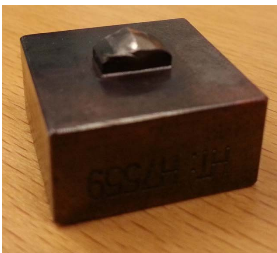
Figure 35: Wedge 120° after testing with increased loading.[2]
