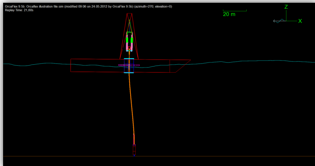
Figure 4.2.6.1: Orcaflex model with JONSWAP waves ( H_S = 3\text{m} )
