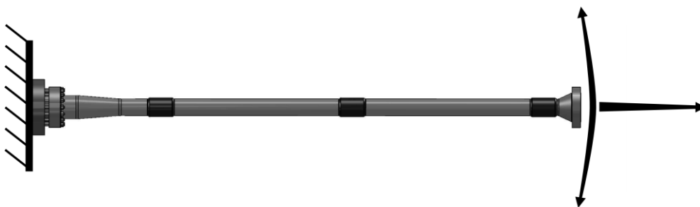
Figure 3.4.2.1: External forces to be applied to prototype through test procedure
