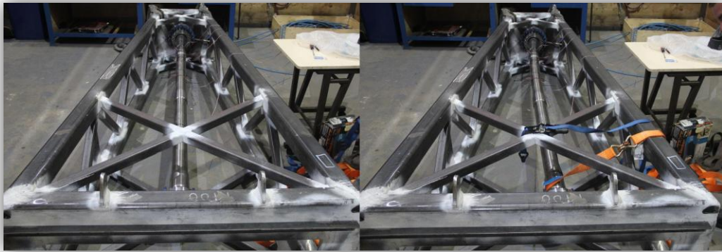
Figure 3.4.8.1: Stage 3 bending of prototype. Max bending at 139,7mm (5,5 inches)
