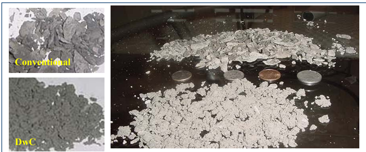
Figure 4.4-Cutting comparison between DwC and conventional drilling [13]
