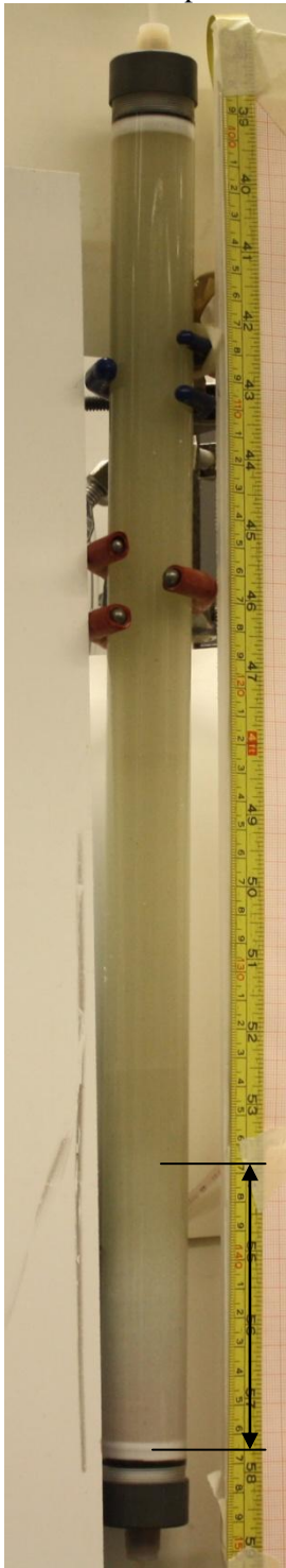
16.03.2010 15:28 Injection of water. White area is viscous fingering. The arrow shows the displacement distance.
