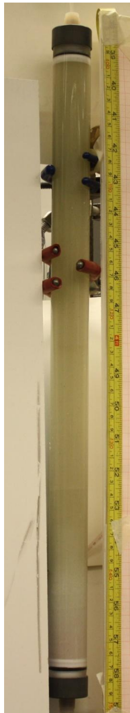
Figure 3-2 Cylindrical test cell
