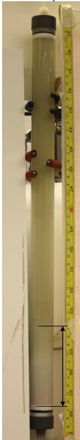
16.03.2010 15:28 Injection of water. White area is probably viscous fingers. The arrow shows the displacement distance.
