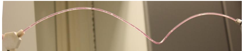
16.03.2010 16:20 Low capillary pressure in the tube
