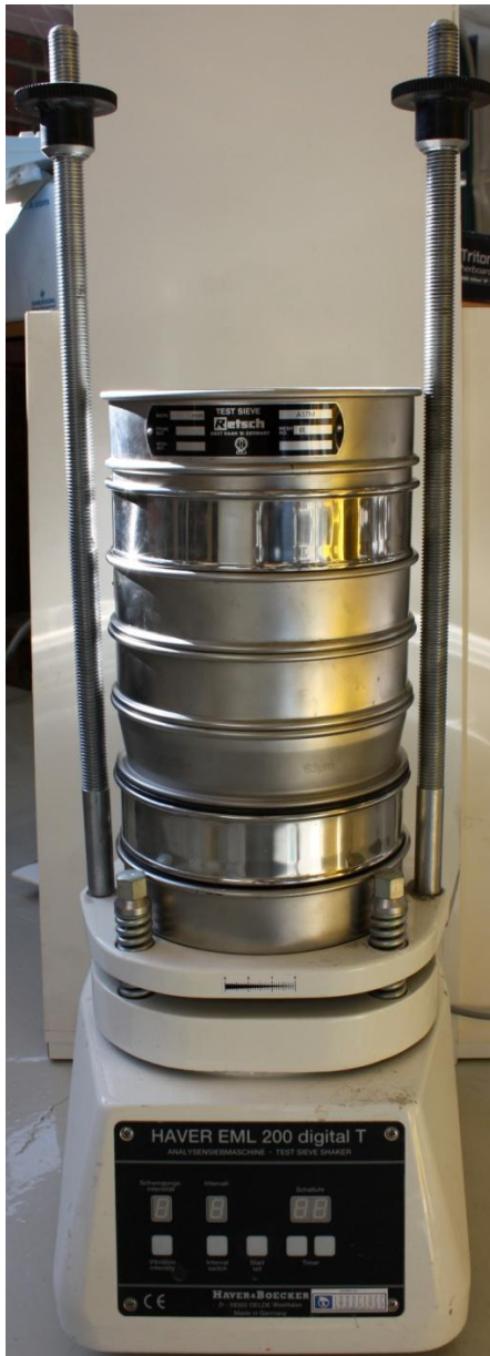
Figure 4-3 Haver EML 200 digital T Test Sieve Shaker used for separation of glass beads
