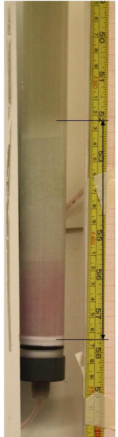
16.03.2010 15:32 Six minutes after injection. Oil displaced 14.2cm in six minutes.
