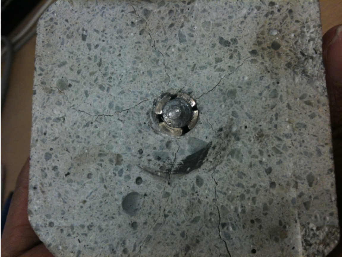
Figure 63: Core showing multiple fractures traveling in different directions
