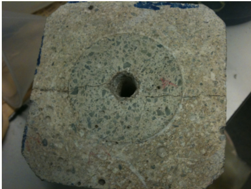
Figure 61: Fracture propagates normal to minimum stress
