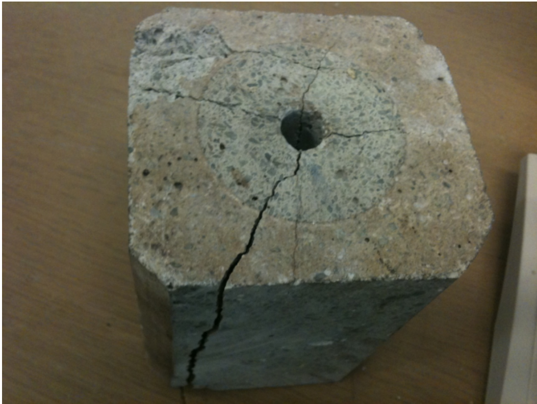
Figure 62: Core showing two fracture directions due to reversed maximum stress
