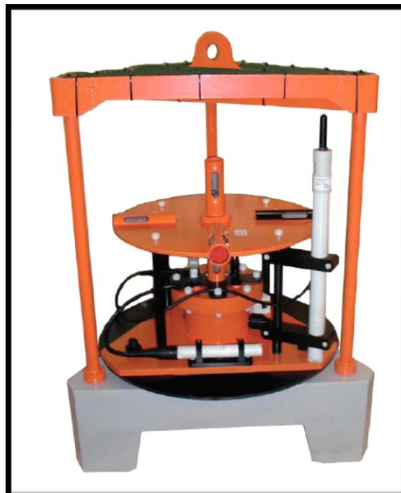
Figure 6.1: UEP sensor frame for installation in the test pit at Nyhamna. (Naxys AS (Frank Sæther), 2011)
