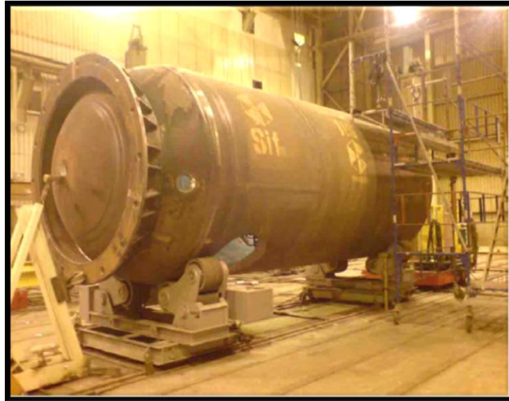
Figure 7.8: The separator vessel during construction. (ShellPictureDatabase, 2011)
