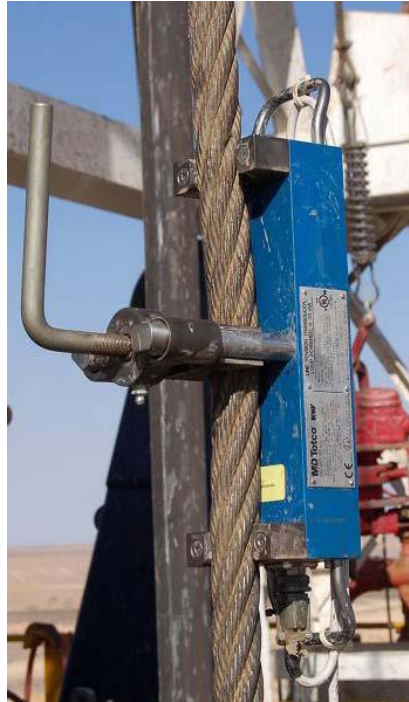
Figure 3.2 Example of bolt on hookload sensor.
