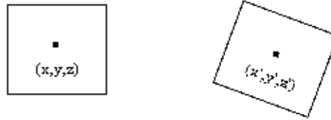
Fig.3.4: A test sample has deformed due to an applied stress, and the position of an arbitrary point inside the sample has shifted
