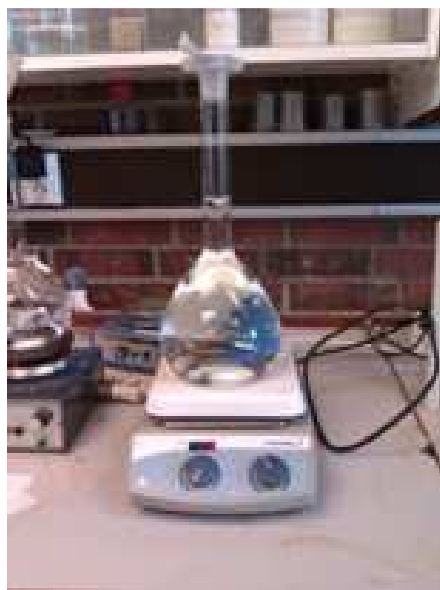
Fig.4.5: The conical flask is placed on a magnetic stirrer. A small magnetic element is placed inside the flask which will rotate due to a alternating magnetic.
