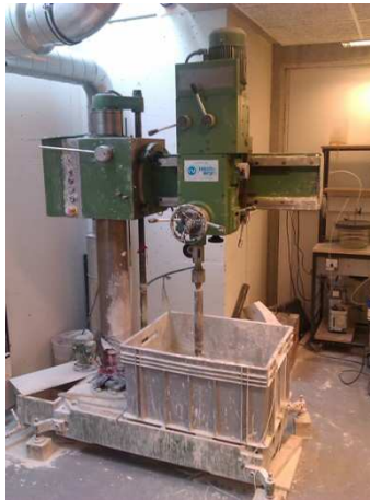
Fig.4.1: Machine used to drill out cylindrical samples from a block of outcrop chalk. Water was used as cooling fluid to prevent the drill bit from overheating.
