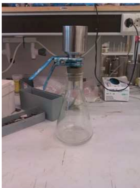
Fig.4.6: Filtrate-apparatus from Millipore used to filtrate the brine. A 0.65\ \mu\text{m} filter was used consistently for all the brine prepared.
