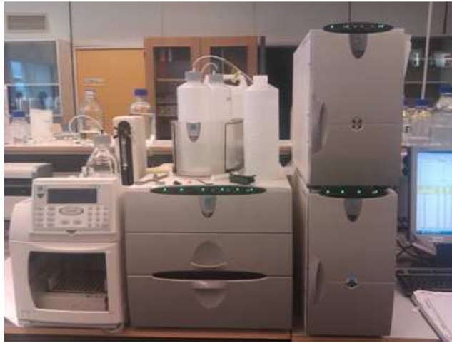
Fig.5.12: A Dionex ICS-3000 ion chromatograph by Dionex Corporation is used to measure the concentration of cations and anions in the effluent samples.
