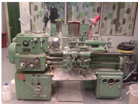
Fig.4.2: The lathe used to reduce the diameter to a predetermined value, to ensure a uniform diameter that will give an isotropic stress field in radial direction during testing.
