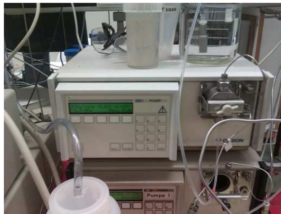
Fig.5.3: Picture of the Gilson 307 pump connected to the flooding line. The pump can pump with a constant flooding rate between 0.010 and 10.0 ml/min. Maximum pressure for this pump is 60 MPa.
