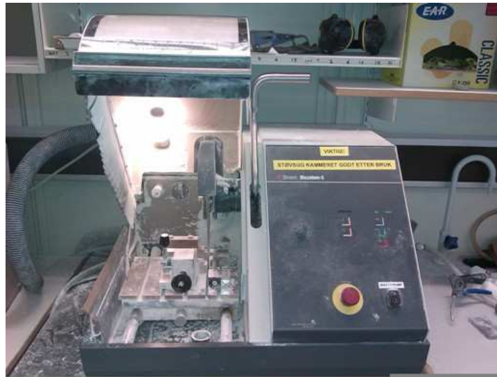
Fig.4.3: Cutting machine used to cut the chalk cores into desired lengths. The cutting machine is equipped with a diamond blade which can cut trough hard materials like flint which often occur in outcrop chalk.
