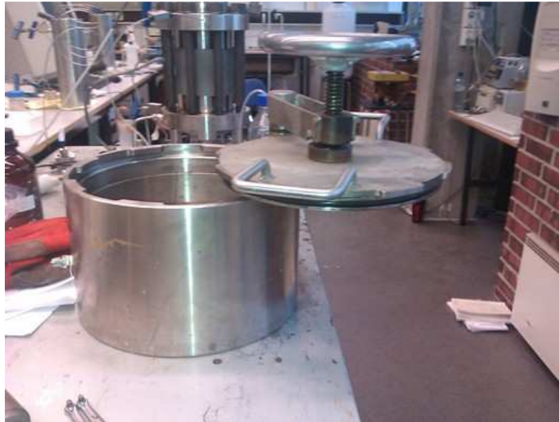
Fig. 4.7: The autoclave used to age cores saturated with both SSW and SSW-(SO 4 2- ) in a heating chamber at 130 °C for three weeks. A back pressure of 0.7 MPa was used to prevent the brine from evaporating.
