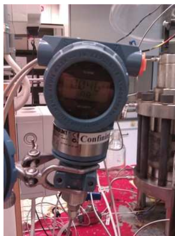
Fig.5.6: Pressure gauge used to monitor confining and piston pressures. Pressure data is sent from the gauges to the logging card on the computer.
