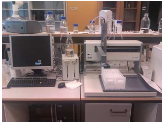
Fig.5.11: A Gilson Gx-271 diluter was used to dilute the effluent samples 200 times. This was done to ensure that the ion concentrations are within the detection range of the IC.
