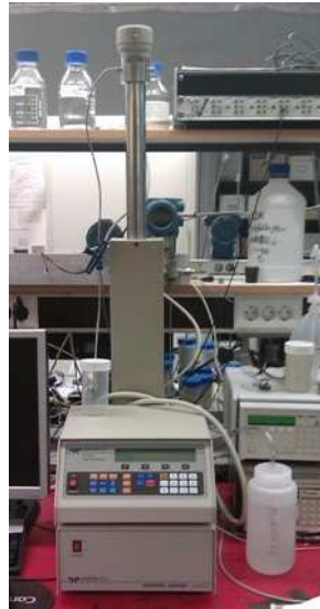
Fig.5.5: Teledyne ISCO 260 D syringe pump used to regulate the back pressure. This type of pump can also pump with constant flooding rate and maintain a constant pressure
