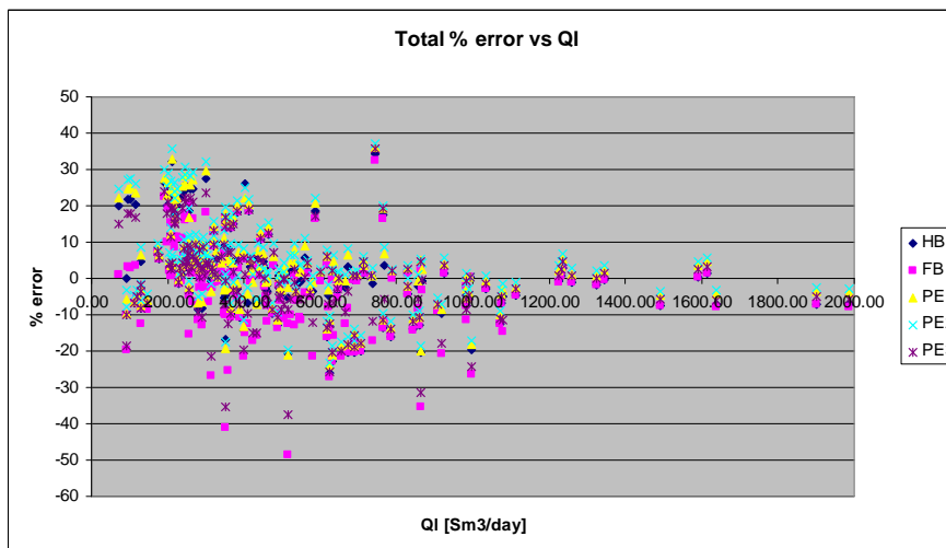
Figure B.52: Percentage error in predicted pressure drop versus liquid rate for all tests
