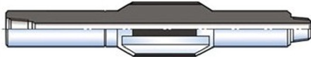
Figure 2.8: Welded blade stabilizer [13].
