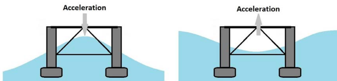
Figure 2.3: A twin pontoon semi-sub on a crest centered wave (left) and a trough centered wave (right). The platform is designed to counteract the passing waves, and is moving opposite to the wave movements.
