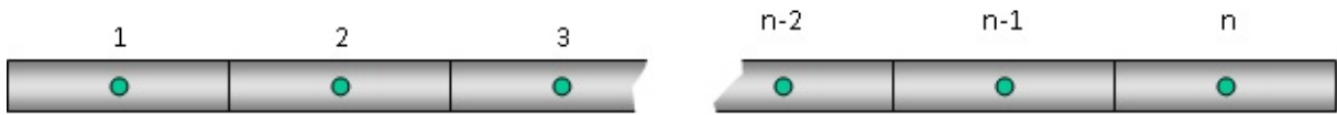
Figure 2.26: A string with free ends having whole segments at both ends. n is the number of segments in the string [21].
