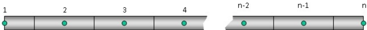
Figure 2.27: A string with free ends having half segments at both ends. n is the number of segment mid points, but the number of whole segments are n-1 [21].
