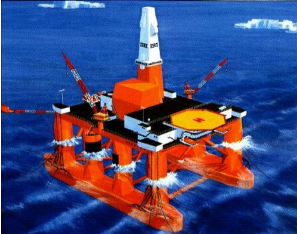
Figure 2.1: A semisubmersible platform with eight columns and two submerged pontoons. The drilling derrick is placed approximately in the middle of the platform [3].
